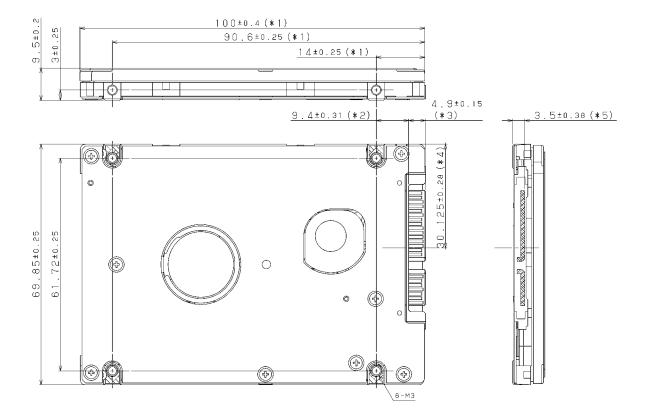
Figure 3.1 illustrates the dimensions of the disk drive. All dimensions are in mm.
